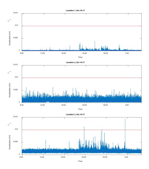
Figure: RMS particle accelerations at Location 1, 2 and 3 on October 16-17, 2017. The magenta dash line represents the mean baseline rms particle acceleration at each location. The red line shows the 0.01 m/s<sup>2</sup> threshold of the rms particle acceleration.
